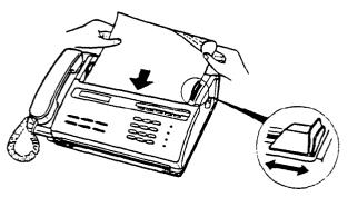
Gently insert the leading edge of the document into the loading slot until you hear a beep tone and the machine has begun to grab the document(s). After the document is secured, the unit displays the standby mode. The document is now loaded and ready to send.
